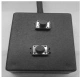
(a) Tpo View of The call and reset switches
